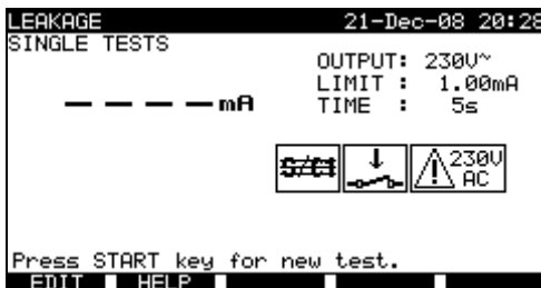
Differential leakage current menu
