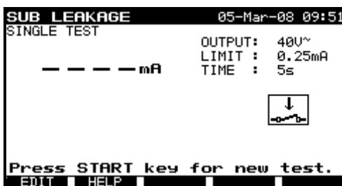
Sub leakage menu
