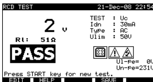
Example of contact voltage measurement results
